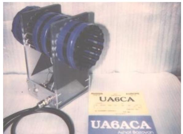
Figure 2 Picture of the Ferrite Magnet Antenna for the 160 and 80- meter Bands
